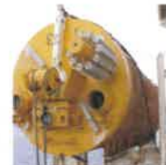
嵌入式拖錨(Drag-embedded Anchor) 吸力式錨(Suction Anchor)
